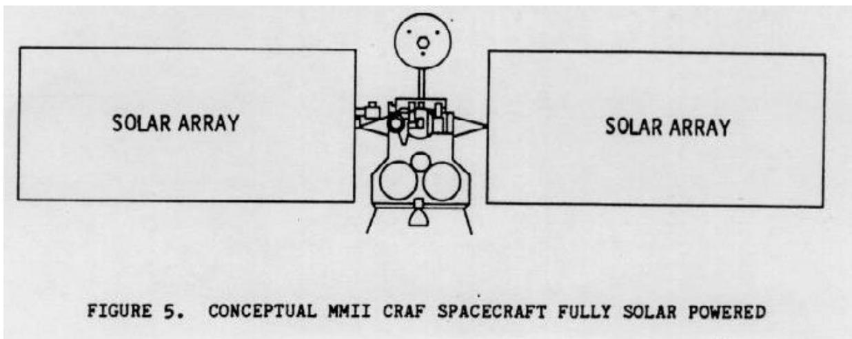
FIGURE 5. CONCEPTUAL MMII CRAF SPACECRAFT FULLY SOLAR POWERED
