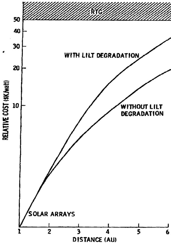
FIGURE 1. SOLAR ARRAY COST vs SOLAR DISTANCE
