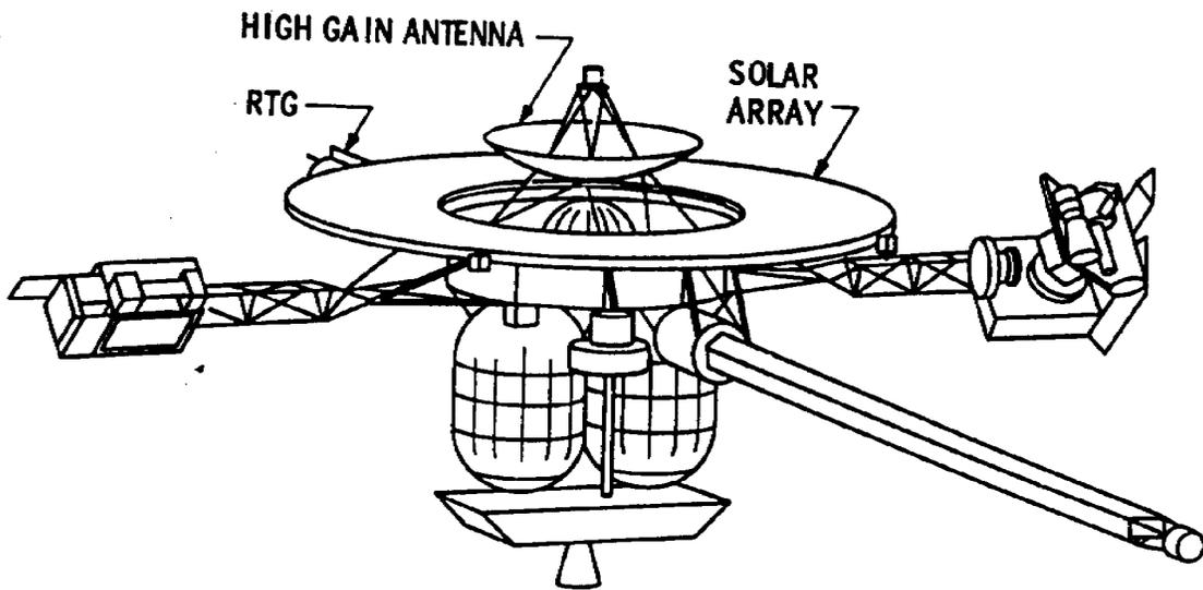
FIGURE 4. ADVANCED CONCEPT SPACECRAFT SOLAR ARRAY CONFIGURATON
